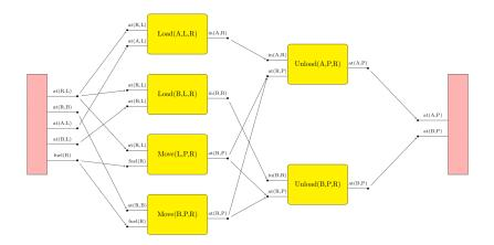
Figure 11: Causal links representing dependencies between actions, connecting preconditions and effects to complete the sequence from the initial state to the goal state.
