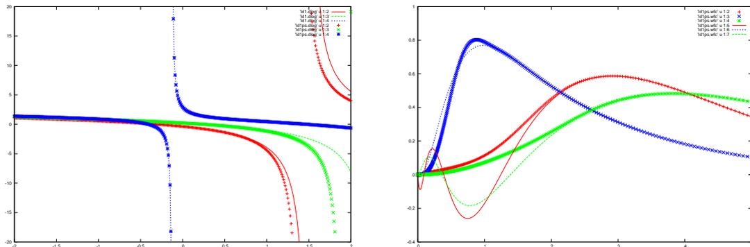
We observe that our PP seems to reproduce fairly well the logarithmic derivatives, with deviations appearing only at relatively high ( $> 1$  Ry) energies. AE and PS orbitals match very well beyond the pseudization radii; the  $3d$  orbital is slightly deformed, because we have chosen a relatively large  $r_c^{(l=2)} = 1.3$  a.u.. It is easy to verify that a smaller  $r_c^{(l=2)}$  yields a better  $3d$  PS orbital, but also a harder  $d$  potential: e.g., for  $r_c^{(l=2)} = 1.0$  a.u., you get
