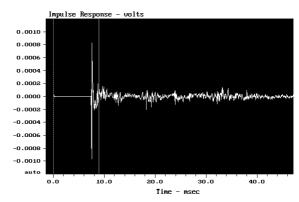
This Impulse Response does not show any strong/dangerous reflections. The FFT of the whole measurement-time (2 sec) does not show any visual signs of coloration:
