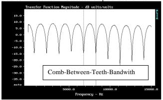
For a single reflection with a time delay of  $\Delta t$  msec, this "Comb-Between -Teeth-Bandwidth is  $1/\Delta t$ .
