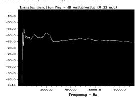
Psycho -acoustic studies (see part 4 +5) indicate that coloration is formed in the first part of the sound. For this sound control-room, it is therefore interesting to investigate the FFT of the direct sound + the first reflection (localised to arrive from the mixing console). Therefore, we will "zoom in" on the part of the Imp. Resp. Before the cursor in the figure above, and perform a FFT for this time window:
