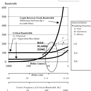
For an orchestra on a platform, Box-Klangfarbe is perceived when a discrete reflection gives a clear combfilter having a "Comb-Between-Teeth-Bandwidth" that is comparable in size to the Critical Bandwidth.
