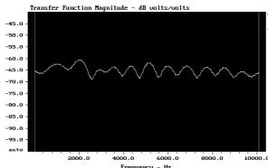
The Comb-Between-Teeth-Bandwidth from this "mixing console-reflection" is some 800 Hz. Examples of other comb-filters are given in the Appendix. (Multiple Reflections etc.) *Are these combfilter "dangerous" concerning coloration?*
